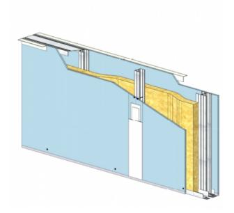
CLOISON SÉPARATIVE KMA 265/125 - KNAUF KA BA18 PHONIK (ACOUSTIQUE) - 18 MM / 18 MM - EI 60 - 65 DB - 5,8M - MONTANT DOUBLE - ENTRAXE 450MM
