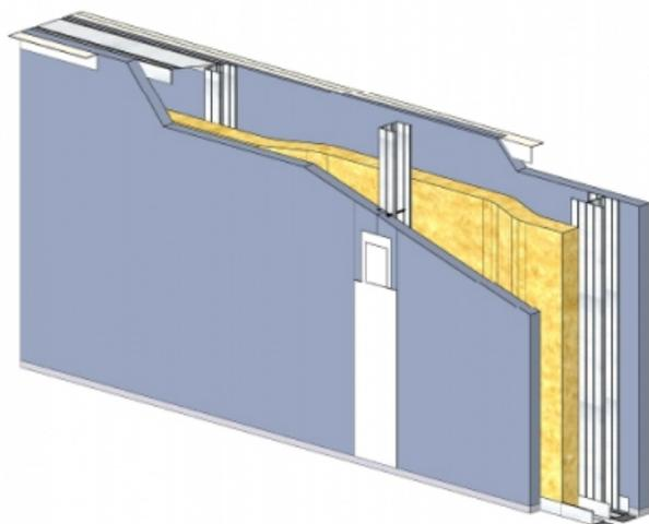
**Cloison séparative KMA 140/48 - KNAUF KA BA25 PHONIK+ (ACOUSTIQUE) - 25 mm / 25 mm - EI 60 - 64 dB - 3,20m - Montant double - Entraxe 900mm**
