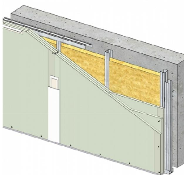
**CONTRE CLOISON CC 318/90 - KNAUF KH-HD BA18/1200 (HYDRO - HAUTE DURETE) - 3X 18 MM - REI 120 - FEU CÔTÉS PLAQUES UNIQUEMENT - 4,55M - MONTANT DOUBLE - ENTRAXE 600MM**
