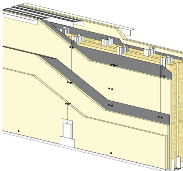
**CLOISON SÉPARATIVE KMA 133/48 - KNAUF SURETE (ANTIEFFRACTION) + KNAUF KS BA13 (STANDARD) - 2X 12,5 MM / 3X 12,5 MM - EI 60 - 60 DB - 3,55M - MONTANT SIMPLE - ENTRAXE 300MM**
