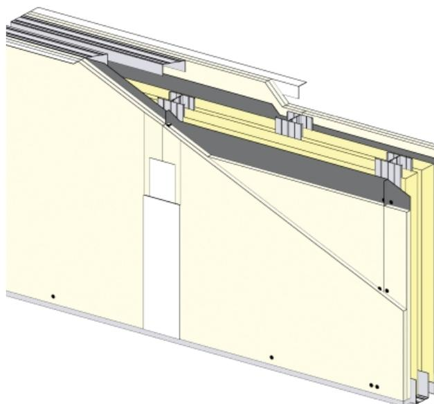
**CLOISON SÉPARATIVE KMA 120/48 - KNAUF SURETE (ANTIEFFRACTION) + KNAUF KS BA13 (STANDARD) - 2X 12,5 MM / 2X 12,5 MM - EI 60 - 45 DB - 3,55M - MONTANT DOUBLE - ENTRAXE 600MM**
